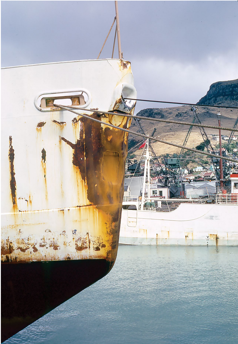
Figure 10.1. The US icebreaker Burton Island in Lyttelton Harbour, February 1973, showing the dent above the belt line after meeting a bergy bit in the Ross Sea.
