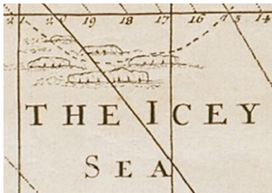
Figure 6.3. Tabular icebergs in the South Atlantic; diagonals are isogonals, connecting points of equal magnetic declination. From Halley's Atlantic chart.
