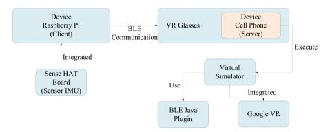
Fig. 9. General architecture of drone-based VR application
