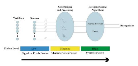
Fig. 10. Sensor fusion system [102].
