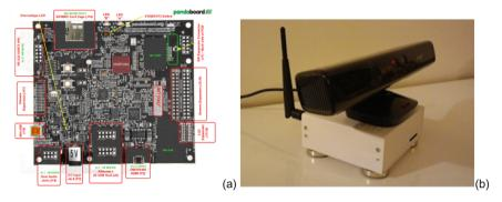
**Fig. 8.** Embedded Kinect Server deployment: Panda board (a) and physical prototype integrated with the MS Kinect for Windows sensor (b)
