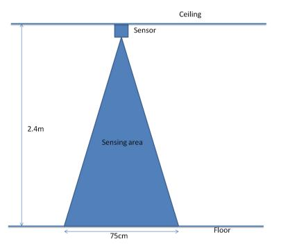
Fig. 8. Example of infrared ceiling sensor network
