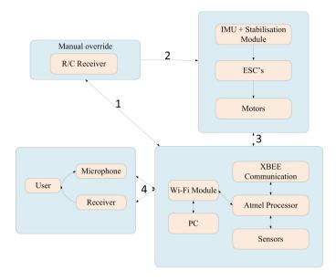
The functional block diagram of Healthbuddy is given in Fig. 8 below.
