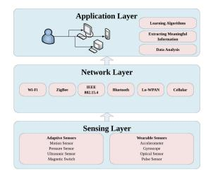
Fig. 3. IoT-based AAL architecture
