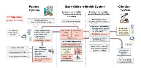
Fig. 3. Overall rehabilitation system architecture
