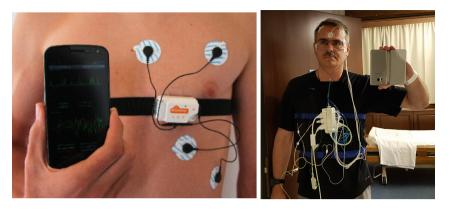
Fig. 6. ECG sensing with Shimmer2R (L) and wearable EEG system (R)
