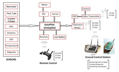
Fig. 1. Basic components of an UAV
