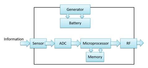
Fig. 6. Monitoring system for data processing
