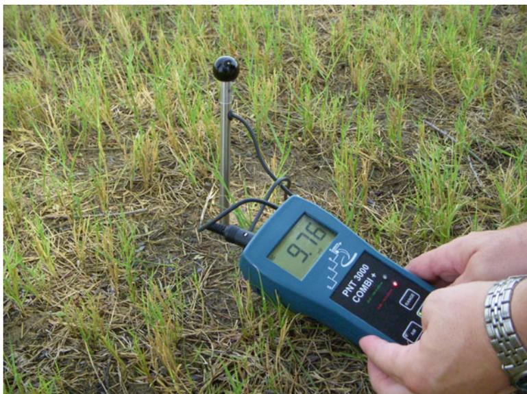
**Plate 1.5** Salinity monitoring in a grass field using salinity probe. (Field scout PNT 3000 COMBI +)
