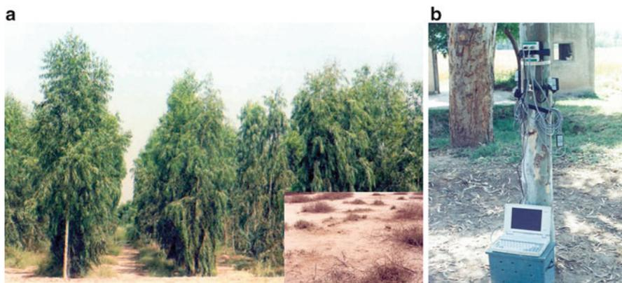
**Plate 3.6** (a) *Eucalyptus camaldulensis* stand on a saline-sodic soil at the Biosaline Research Station of NIAB (Pakka Anna), near Faisalabad, monitored for tree water use with HeatPulse Data Loggers. (Adapted from Mahmood et al. 2004), (b) Setup for monitoring tree water use with HeatPulse Technique
