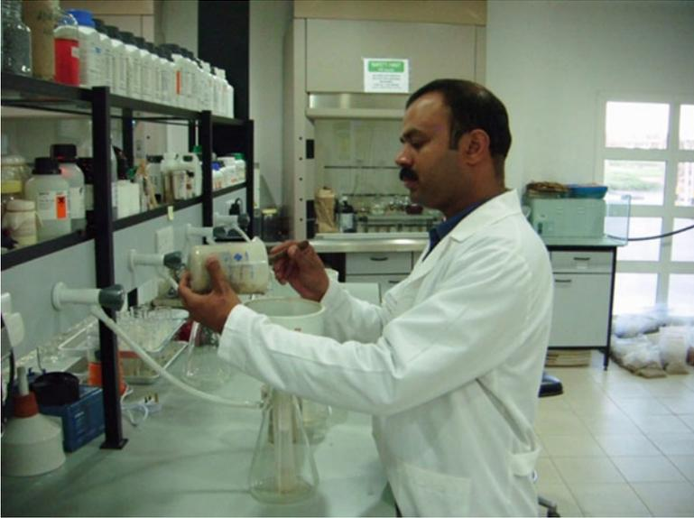
**Plate 1.4** Setup for collection of extract from saturated soil paste
