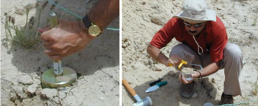
**Plate 3.2** Collection of a soil core to measure bulk density of the soil, and cleaning the core with a saw
