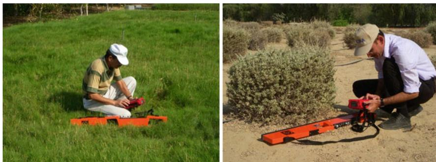
**Plate 1.6** EC measurement with EM 38 in vertical mode (left: grassland) and horizontal mode (right: *Atriplex* field)
