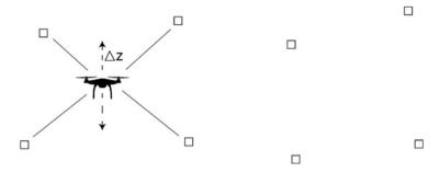
**Fig. 6** Example setup in which anchors are visualised as squares. The additional distance measurements between tag and anchors during a short reference flight, varying the z value of the tag, are visualised as lines. Source: own elaboration
