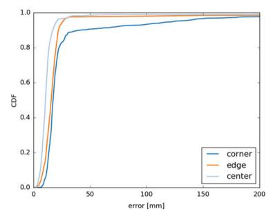
Fig. 4 CDF of drone positioning error for three different key locations in the convex hull of anchors. Source: own elaboration
