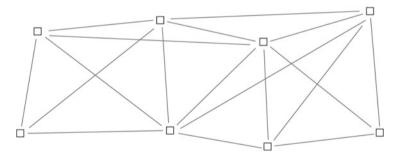
Fig. 5 Example setup in which anchors are visualised as squares. The lines connecting them represent the measured inter-anchor distances, to be used in auto-calibration. Source: own elaboration
