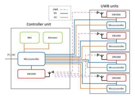
Fig. 1 Adapted high-level overview of the system on the drone. Source: own elaboration
