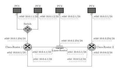
Fig. 5. Typical infrastructure setup within the iLab course
