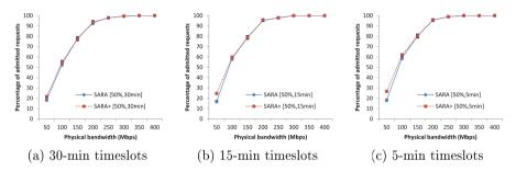
Fig. 5. Impact of timeslot size with 50% backup demand in the timeslot-based advance bandwidth reservation approach.
