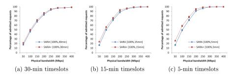
Fig. 4. Impact of timeslot size with 100% backup demand in the timeslot-based advance bandwidth reservation approach.
