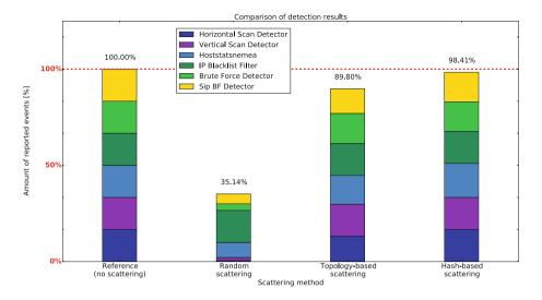
**Fig. 6.** Comparison of the detection results after applying various scattering methods. Each part of column with different color stands for normalized number of unique events reported by different detection method. (Color figure online)
