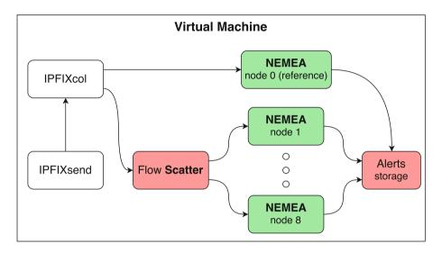
Fig. 4. Testing environment for experiments and evaluation of various methods of flow data distribution between computational nodes running flow-based NIDS NEMEA.
