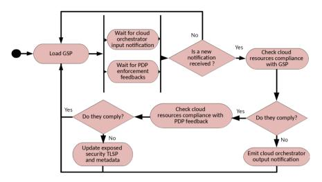
Fig. 3. Overview of the security orchestrator activity diagram
