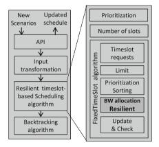
Fig. 1. Components of the resilient advance bandwidth reservation approach.
