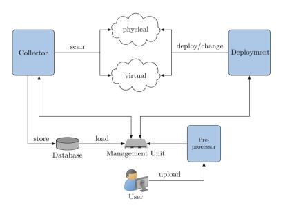
Fig. 1. System overview of INSALATA showing basic components
