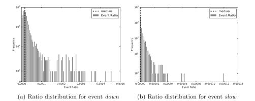
Fig. 2. Event ratios of the analyzed data set. The right most spikes, that constitute a multiple of the average ratio, are related to Amazon's S3 outage during the capture time of the data set.
