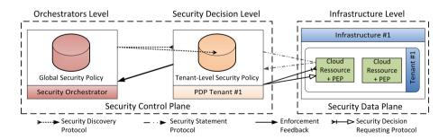
Fig. 1. SDSec framework in a single-infrastructure single-tenant scenario
