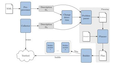
Fig. 4. Execution flow of INSALATA's Deployment Component
