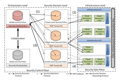
**Fig. 2.** SDSec framework interacting with a cloud orchestrator, in a multi-cloud multitenant scenario. (1) accounts for the TLSP fetching, (2) for the security statement, (3) for the enforcement feedback and (4) for the policy decision request.
