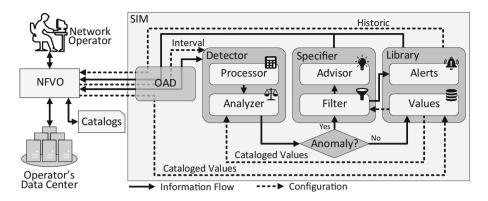
**Fig. 1.** Detailed SIM architecture [2] – The SIM communicates directly with NFVOs, using standard northbound APIs for requesting information regarding NFV elements operation and also to forward the results of the anomaly detection analysis.
