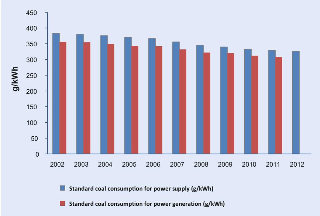
■ Fig. 3.2 Standard coal consumption (2002–2012), data from [10]
