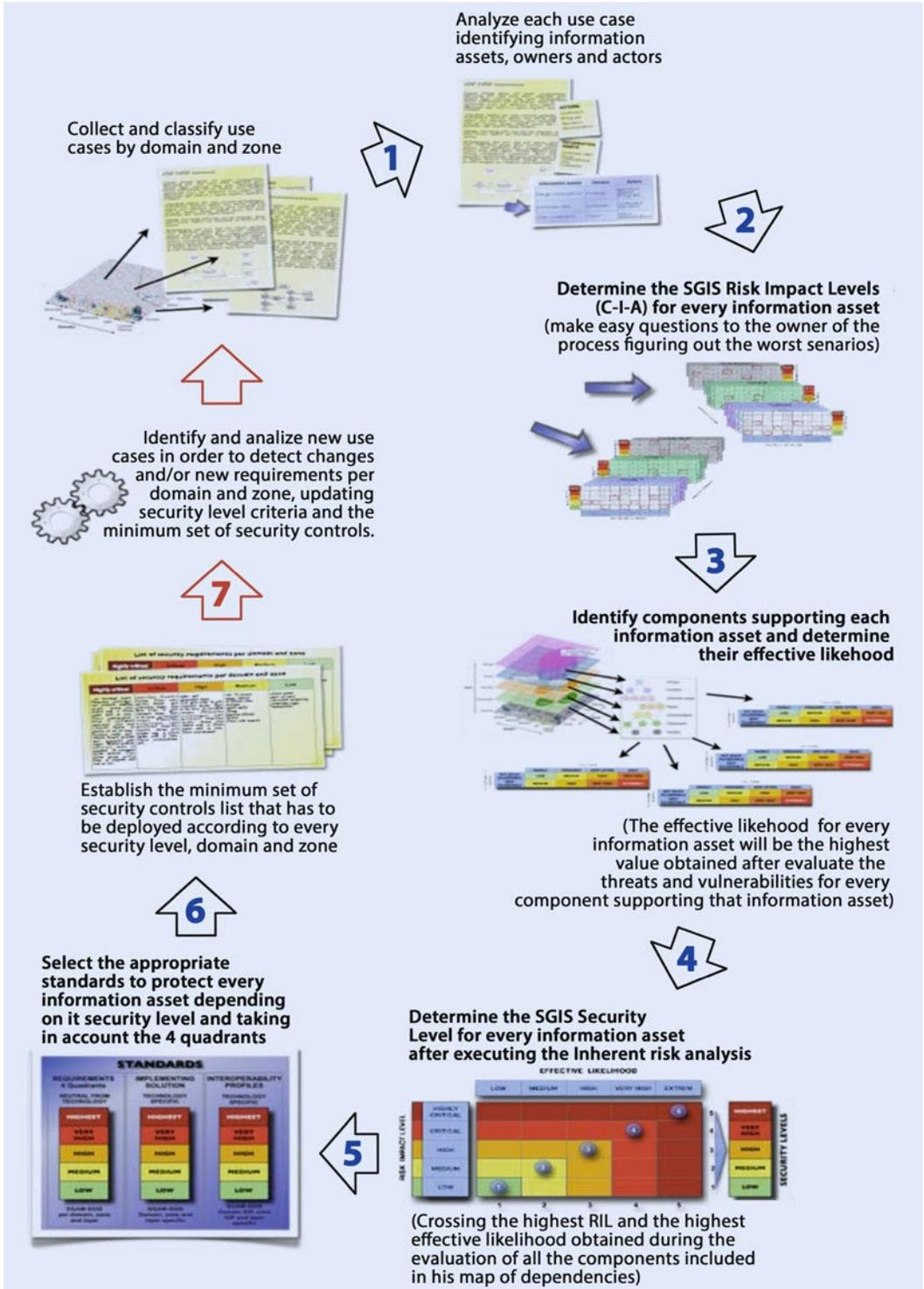
Fig. F.2 Overview on the smart grid security assessment proposed by WG SGIS, taken from [1]
