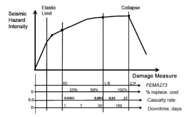
**Fig. 3.7** Conceptual relationship between seismic hazard intensity and structural performance (From Krawinkler and Miranda (2004), courtesy W. Holmes, G. Deierlein)
