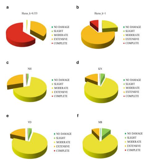
**Fig. 3.19** Seismic risk (physical damages) in SCD16 for Hazard 3 and mean return period of 475 years in terms of the percentage of damage per damage state using (**a**) ATC-40 methodology combined with Hazus for k = 0.333 (**b**) ATC-40 methodology combined with Hazus for k = 1 (**c**) Newmark and Hall (1982) (**d**) Krawinkler and Nassar (1992) (**e**) Vidic et al. (1994) and (**f**) Miranda and Bertero (1994)
