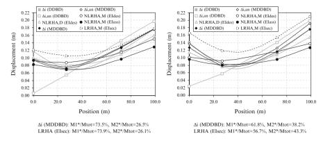
Fig. 7.12 Nonlinear response history maximum displacements for evaluation cases NLRHA (EIdes), (EIass) and linear response history maximum displacements for evaluation case NLRHA(EIdes). *Left*: Zone II; *Right*: Zone III, compared with target-displacements profiles ( $\Delta$ i) and displacement profiles obtained from structural analyses ( $\Delta$ i,an) according to DDBD (D) and Modal DDBD (M)
