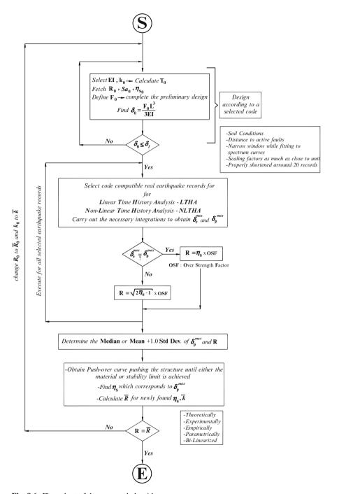
Fig. 8.6 Flow chart of the proposed algorithm
