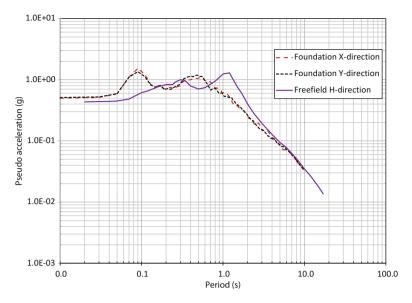
Fig. 6.7 Kinematic interaction motion for "stiff" piled foundation 1
