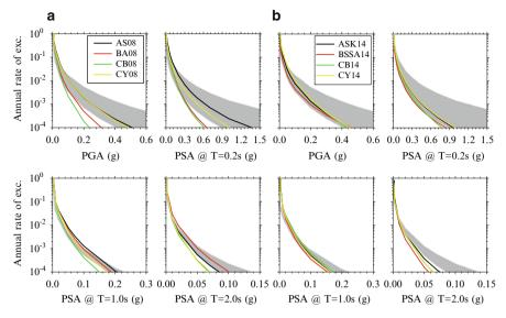
Fig. 12.18 Same as Figs. 12.14 and 12.16 but comparisons are between (a) NGA-West1 vs. pan-European GMPEs and (b) NGA-West2 vs. pan-European GMPEs for moderate-seismicity region
