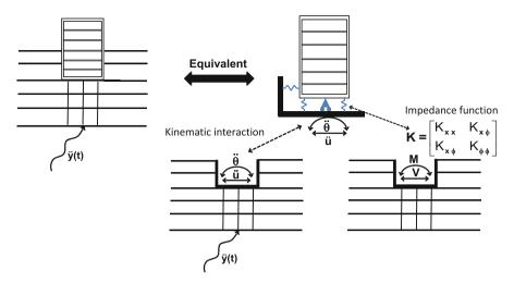
Fig. 6.4 Substructuring approach for soil structure interaction
