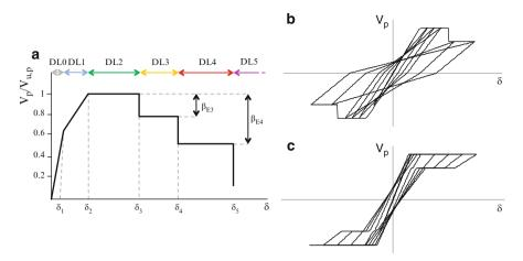
**Fig. 11.2** Backbone of a masonry panel based on a multilinear constitutive law (Adapted from Cattari and Lagomarsino (2013)) (a) and sketch of some typical hysteretic responses of masonry piers subjected to a prevailing shear (b) and flexural (c) failure mode
