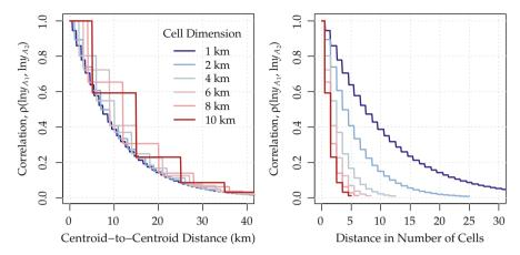
Fig. 4.18 Example correlations computed using Eq. (4.29) for square cells of differing dimension
