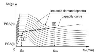
Fig. 7.11 Capacity and demand spectra
