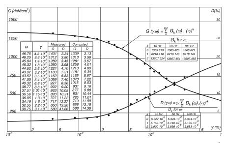
**Fig. 17.3** The absolute values of the variation of dynamic torsion modulus function  $(G, \text{daN/cm}^2)$  and torsion damping function (D %) of specific strain  $(\gamma \%)$  for marl samples obtained in Hardin and Drnevich resonant columns from NIEP (USA patent), Laboratory of Earthquake Engineering (Marmureanu et al. 2010)
