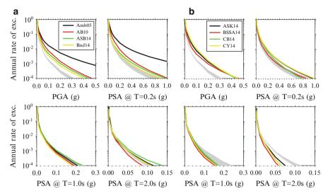
Fig. 12.14 Comparisons of hazard curves for PGA, PSA at T=0.2s, T=1.0s and T=2.0s between (a) Turkish vs. pan-European GMPEs and (b) Turkish vs. NGA-West2 GMPEs for the chosen moderate-seismicity region
