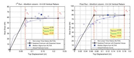
**Fig. 8.11** Comparison of the assumed capacity curve with the pushover and time history analyses results for the Column #2
