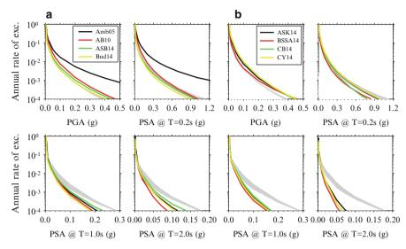
**Fig. 12.16** Same as Fig. 12.14 but the comparisons are between (a) Italian vs. pan-European GMPEs and (b) Italian vs. NGA-West2 GMPEs for moderate seismicity
