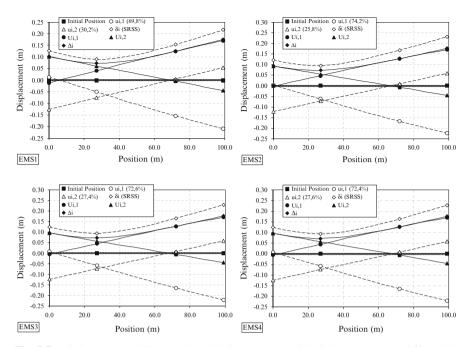
Fig. 7.7 Displacement profiles: Peak modal displacements ui,j, displacement pattern  $\delta i$ , modal target-displacement profiles Ui,j and target-displacement profiles  $\Delta i$ , derived iteratively from the EMS method
