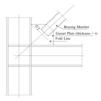
Fig. 5.10 Gusset plate connections in concentrically braced frames
