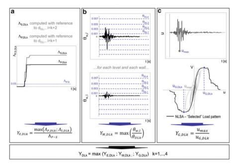
**Fig. 11.6** Multiscale approach for the DLs identification in case of NLDA (for a given time history as scaled to a given intensity measure, in the case of IDA method). (a) Element scale. (b) Macroelement scale. (c) Global scale
