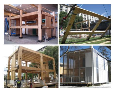
**Fig. 13.29** From laboratory specimen to office building: 3D Test Specimen tested in the lab (Newcombe et al. 2010), demounted and reconstructed (Smith et al. 2011) on UC campus as EXPAN/STIC office
