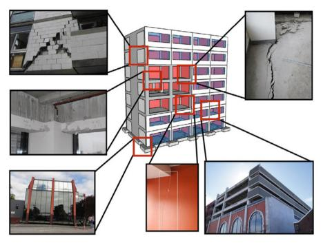
**Fig. 13.6** Holistic representation of damage/performance to a modern building, including structural skeleton (frame system, floor diaphragm), non-structural components (lightweight partitions, heavy brick infills and precast concrete facades) and foundation system (significant settlements and residual tilting) (Modified after Johnston et al. (2014))
