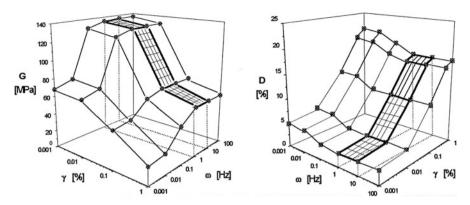
**Fig. 17.7** Dependence of dynamic torsion modulus function  $(G, \text{daN/cm}^2)$  and torsion damping function (D%) with shear strains  $\gamma\%$  and frequency  $\omega$ . For frequencies between 1 and 10 Hz, shear modulus (G) and damping ratio are constant in this main field used in engineering (Bratosin 2002; Marmureanu et al. 2005, 2010, 2013)
