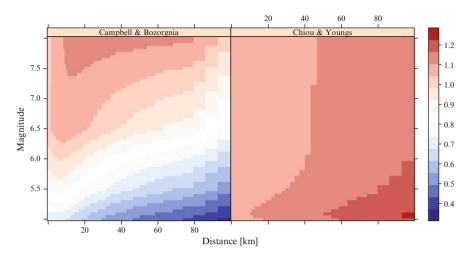
**Fig. 4.2** Example *bias factors* computed as the ratios between predictions of two generations of models from the same developers. The *left* panel shows ratios between the medians, Sa(T=0.01s), of Campbell and Bozorgnia (2014, 2008) – 2014:2008, while the *right* panel is for Chiou and Youngs (2014, 2008) – 2014:2008
