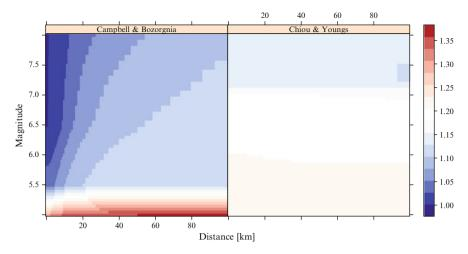
**Fig. 4.3** Example *bias factors* for the logarithmic standard deviations. The *left* panel shows ratios between the  $\sigma_{\ln Sa}$  predictions of Campbell and Bozorgnia (2014, 2008) – 2014:2008, while the *right* panel shows the ratios for Chiou and Youngs (2014, 2008) – 2014:2008. The standard deviations are for a period of 0.01 s
