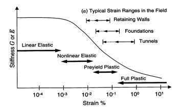
**Fig. 17.2** Stiffness degradation curve in terms of shear modulus G and Young's modulus E: stiffness plotted against logarithm of typical strain levels observed during construction of typical geotechnical structures (Marmureanu et al. 2013)
