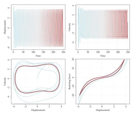
Fig. 4.11 Response of the nonlinear system for a harmonic amplitude of B = 5. Upper left panel shows the displacement time-history; upper right panels shows the velocity time history; lower right panel shows the response trajectory in phase space; and lower right panel shows the hysteretic response
