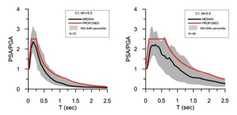
**Fig. 3.4** Normalized elastic acceleration response spectra for soil class C1 of the classification system of Pitilakis et al. (2013) for Type 2 seismicity (*left*) and Type 1 seismicity (*right*). *Red lines* represent the proposed spectra. The range of the 16th to 84th percentile is illustrated as a gray area
