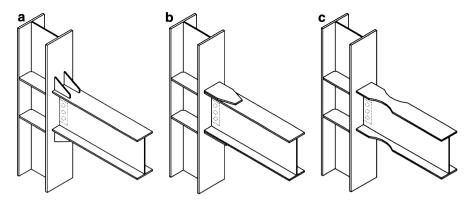
Fig. 5.9 Examples of modified moment beam-to-column connection configurations: (a) with haunches, (b) with cover plates; (c) reduced beam section
