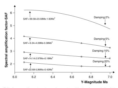
Fig. 17.11 Strong nonlinear dependence of spectral amplification factors (SAF) of Vrancea earthquake magnitude on extra-Carpathian area (Marmureanu et al. 2013). Magnitude  $M_S$  is on Richter scale (Marmureanu et al. 2010)
