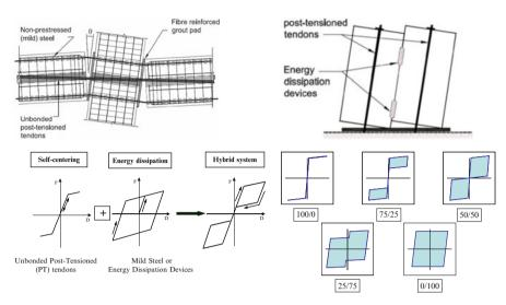
**Fig. 13.7** *Top*: Jointed precast "hybrid" frame and wall connections developed in the US PRESSS-Program (*fib* 2003; NZS 3101:2006, NZCS 2010. *Bottom*: flag-shape hysteresis loop for a hybrid system (modified after *fib* (2003)) and effects of varying the ratio between re-centering vs. dissipative contribution (courtesy of Nakaki and Stanton)
