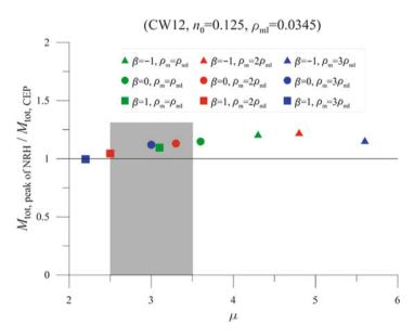
**Fig. 9.8** Total base overturning moment capacity obtained from NRHA divided by the same from proposed procedure versus ductility demand (CW12,  $n_0 = 0.125$ , Chi-chi earthquake – record no: TCU065)
