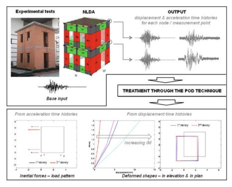
Fig. 11.4 Sketch on the use of POD technique to process data from experimental tests or NLDA results (Data adapted from Cattari et al. (2014))
