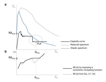
Fig. 11.9 CSM procedure proposed for the evaluation of  $\rm IM_{PL}$  in case of capacity curves characterized by sudden base shear decay
