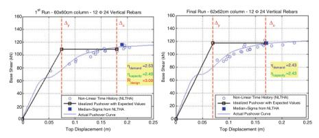
**Fig. 8.10** Comparison of the assumed capacity curve with the pushover and time history analyses results for the Column #1
