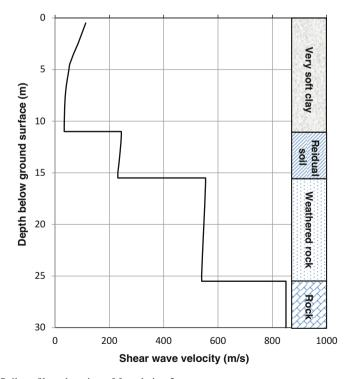
Fig. 6.6 Soil profile at location of foundation 2
