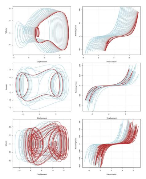
**Fig. 4.13** Response of the nonlinear system for a harmonic amplitude of B = 15 (top), B = 35 (middle), and B = 65 (bottom). Panels on the left show the response trajectory in phase space; and panels on the right show the hysteretic response
