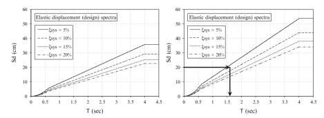
**Fig. 7.4** Elastic displacement response spectra for various damping ratios; *left*: Zone II (PGA = 0.24 g), *right*: Zone III (PGA = 0.36 g)
