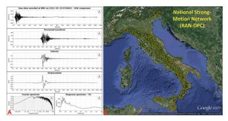
Fig. 2.6 (a) waveforms extracted from ITACA database, and (b) geographical distribution of the National Strong-Motion Network (RAN-DPC)
