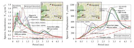
**Fig. 13.2** Acceleration and Displacement response spectra from 4 records in the CBD of the 22nd Feb 2011 event, compared with the code design spectra (NZS1170:5 2004) *thick red line* = 1/2,500 years event (MCE); *red line* = 1/500 years event (DBE) (Kam and Pampanin 2011)
