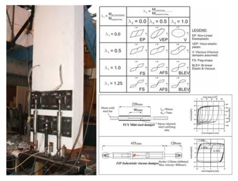
**Fig. 13.11** Concept, implementation and experimental validation (*shake-table*) of the concept of Advanced Flag-Shape applied to a post-tensioned wall (Kam et al. 2010; Marriott et al. 2008, 2009). Combination in parallel of hysteretic and viscous dampers
