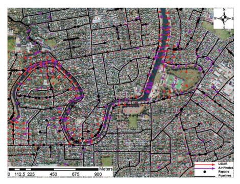
Fig. 10.5 Ground displacement from LiDAR and air photos superimposed on pipelines and pipe repairs in Avonside (Toprak et al. 2014)
