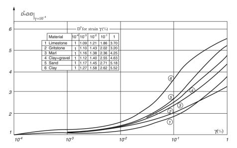
**Fig. 17.6** Nonlinear relation between torsion damping function (D%) and shear-strain ( $\gamma\%$ ) experimental data from Hardin and Drnevich resonant columns from NIEP (USA patent). Normalized values for limestone, gritstone, marl, clay+gravel, sand, and clay (Marmureanu et al. 2010)
