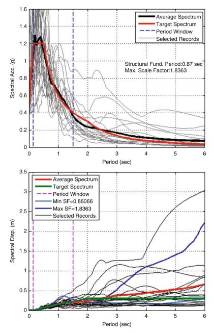
Fig. 8.5 Acceleration spectra and displacement spectra for an example selection
