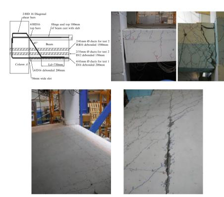
Fig. 13.17 "Non tearing floor" or top-hinge solution: *Top left*: schematic (*left*, Muir et al. 2013) and comparison of damage to plastic hinges (*Top centre and right*) and to the floor (*bottom left and right*) from the testing of a 3-D superassemblage implementing a top-hinge solution (*top centre and bottom left*, Muir et al. 2012) vs. a traditional beam-column connection (*top right* from MacPherson 2005, *bottom right*, Lindsay 2004)
