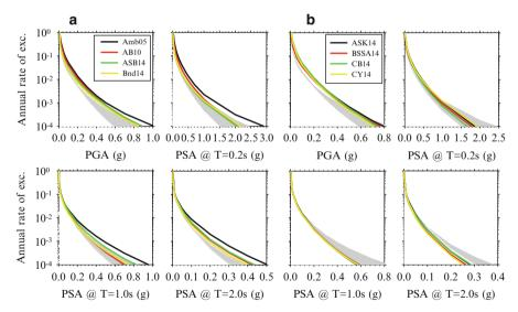
Fig. 12.15 Comparisons of hazard curves for PGA, PSA at T=0.2s, T=1.0s and T=2.0s between (a) Turkish vs. pan-European GMPEs and (b) Turkish vs. NGA-West2 GMPEs for the chosen high-seismicity region
