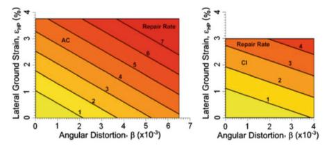
Fig. 10.7 Repair rate vs lateral strain, and angular distortion for AC and CI pipelines (O'Rourke et al. 2014)
