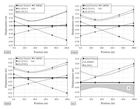
Fig. 7.5 Displacement profiles (EMS): Peak modal displacements  $u_{i,j}$ , displacement pattern  $\delta_i$  and target-displacement profiles  $\Delta_i$ , estimated iteratively from the EMS method. Structural analysis displacement profile (SA1) compared with target-displacement profile (inertia forces  $(F_i)$  on the MDOF structure also illustrated)
