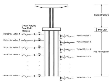
Fig. 6.1 Global pile-structure model
