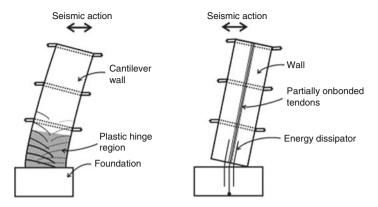
**Fig. 13.8** Comparative response of a traditional monolithic system (damage in the plastic hinge and residual deformations) and a jointed precast (hybrid) solution (rocking mechanism with negligible damage and negligible residual deformations *fib* 2003)
