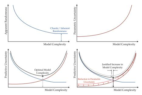
**Fig. 4.15** Schematic illustration of the trade-off that exists between the reduction in apparent randomness (*upper left*) and the increase in parametric uncertainty (*upper right*). The optimal model in this context balances the two components (*lower left*) and an increase in complexity is justified when parametric uncertainty is reduced (*lower right*)
