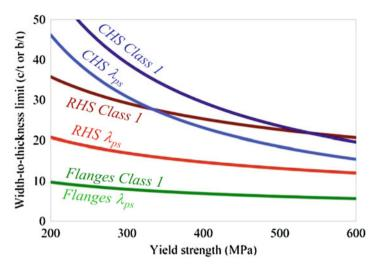
Fig. 5.1 Comparison of width-to-thickness requirements for high ductility
