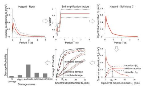
Fig. 3.9 Schematic example of estimated damages when using the median for UHS for rock, soil amplification factors, capacity curve and fragility curves
