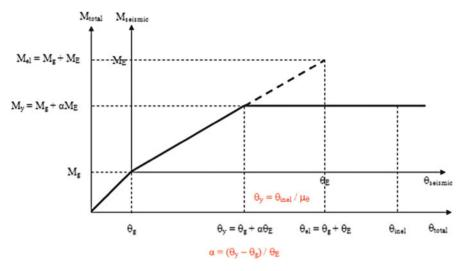
Fig. 7.10 Definition of the correct slope of M-  $\theta_{inel}$  diagram and of  $a\theta_{E}$
