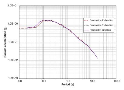
Fig. 6.5 Kinematic interaction motion for "flexible" piled foundation 1
