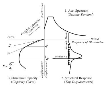
Fig. 8.7 Description of the proposed procedure
