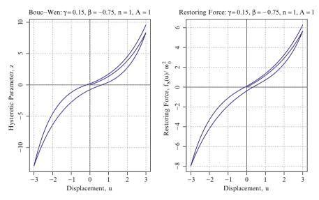
**Fig. 4.10** Dependence of the hysteretic parameter z (*left*), and the normalised restoring force  $f_S$  ( $u, \dot{u}, z$ ) (right) on the displacement for the example system considered
