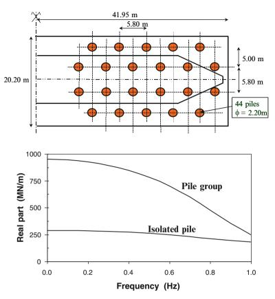
Fig. 6.3 Horizontal pile group impedance for the Vasco da Gama bridge (Pecker 2003)
