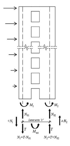
The base section of the coupled core wall system is the most critical section controlling the nonlinear behaviour of the entire structure. Total base overturning moment reaction of the coupled wall system can be expressed by the following equilibrium equation:
