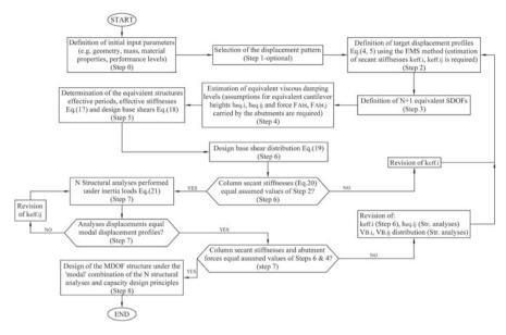
Fig. 7.1 Modal direct displacement-based design of bridges
