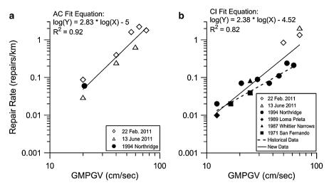
Fig. 10.1 Repair rate vs. GMPGV for (a) AC pipelines and (b) CI pipelines (O'Rourke et al. 2014)
