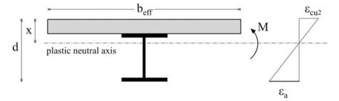
Fig. 5.3 Ductility and effective width of composite beam sections
