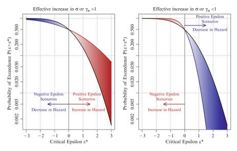
**Fig. 4.1** Illustration of the effect that a bias in the logarithmic standard deviation has upon the computation of probabilities of exceedance. The *left* panel corresponds to  $\gamma_{\sigma} = 2$  while the *right* panel shows  $\gamma_{\sigma} = 1/2$
