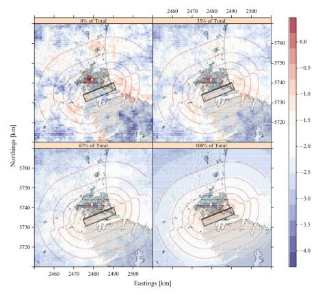
**Fig. 4.7** Impact upon the nature of ground-motion fields generated assuming that the inter-event variability is a given fraction of the total aleatory variability. The ground-motion fields shown are possible fields consistent with a repeat of the Christchurch earthquake
