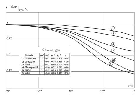
**Fig. 17.5** Nonlinear relation between dynamic torsion modulus  $(G, \text{daN/cm}^2)$  and shear-strain  $(\gamma\%)$  experimental data from Hardin and Drnevich resonant columns from NIEP (USA patent). Normalized values for limestone, gritstone, marl, clay+gravel, sand, and clay (Marmureanu et al. 2010)
