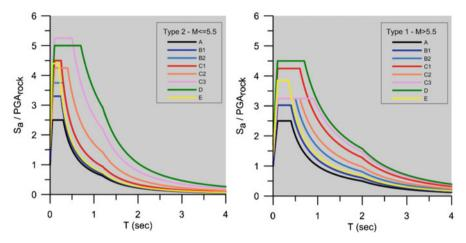
**Fig. 3.5** Type 2 (*left*) and Type 1 (*right*) elastic acceleration response spectra for the classification system of Pitilakis et al. (2013)
