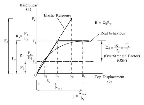
Fig. 8.13 The use of equal displacement rule in design
