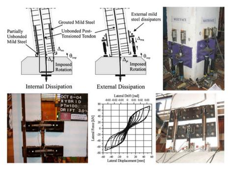
**Fig. 13.10** *Top*: Internal vs. external replaceable dissipaters/fuses in a column/pier. *Bottom*: Alternative configuration of Plug&Play dissipaters for bc joints or walls (Marriott et al. 2008, 2009, 2010)
