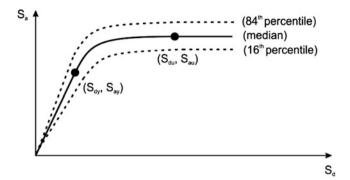
Fig. 3.16 Typical capacity curve in EQRM software, defined by the yield point  $(S_{dy}, S_{ay})$  and the ultimate point  $(S_{du}, S_{dy})$  (Modified after Robinson et al. (2005))
