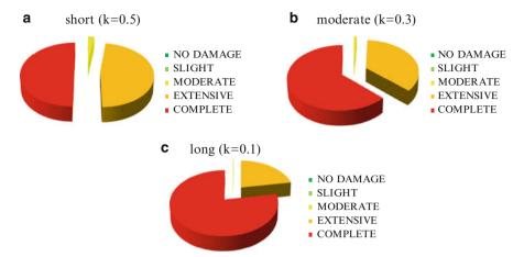
**Fig. 3.20** Computed damages for SCD16 for Hazard 3 and mean return period of 475 years in terms of the percentage of damage per damage state considering (**a**) short (**b**) moderate and (**c**) long duration of the ground shaking
