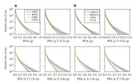
**Fig. 12.19** Same as Figs. 12.15 and 12.17 but comparisons are between (a) NGA-West1 vs. pan-European GMPEs and (b) NGA-West2 vs. pan-European GMPEs for high-seismicity region
