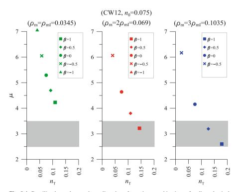
Fig. 9.4 Ductility demand vs total coupling shear for various combinations of wall mechanical reinforcement ratio and relative yield parameter (CW12,  $n_0 = 0.075$ )
