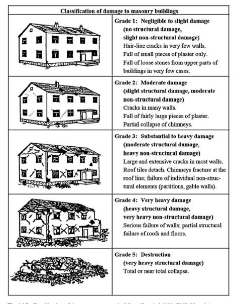
Fig. 16.3 Classification of damage to masonry building (Grünthal 1998, EMS-98 scale)
