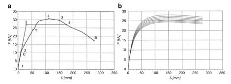
**Fig. 8.9** Determination of the column capacity curve (a) Bilinear idealization of capacity curve (b) Effect of longitudinal reinforcement ratio on the capacity curve
