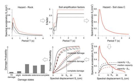
Fig. 3.10 Schematic example of estimated damages when using the median  $\pm 1$  standard deviation (depending on which one is the more "conservative" or reasonable) for UHS for rock, soil amplification factors, capacity curve and fragility curves
