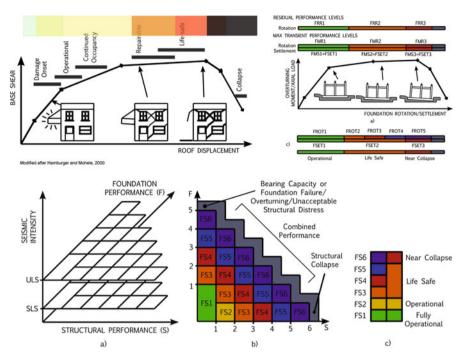
**Fig. 13.23** Concept of a performance matrix (*bottom*) for integrated structure-foundation design combining limit states for structure (*top left*) and foundation (*top right*) (Giorgini et al. 2014)
