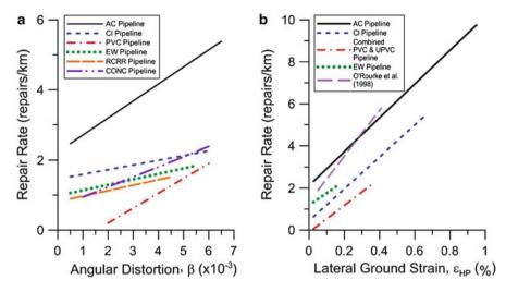
Fig. 10.6 Comparison of repair rate vs. angular distortion and lateral strain for different pipe types (O'Rourke et al. 2014)
