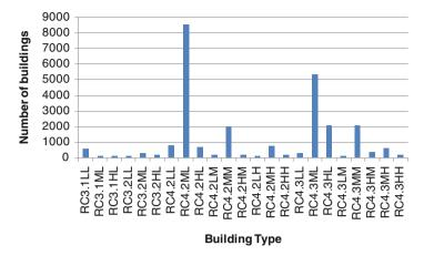
Fig. 3.15 Classification of the RC buildings of the study area (Kappos et al. 2006). The first letter of each building type refers to the height of the building (L low, M medium, H high), while the second letter refers to the seismic code level of the building (N no, L low, M medium, H high)
