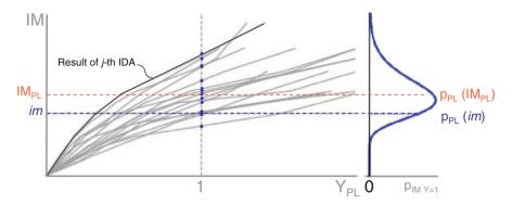
Fig. 11.10 Results of IDA and evaluation of IM<sub>PL</sub>
