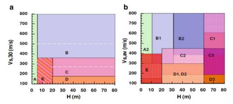
Fig. 3.3 Simplified illustration of ground types according to (a) EC8 and (b) the new classification scheme of Pitilakis et al. (2013)
