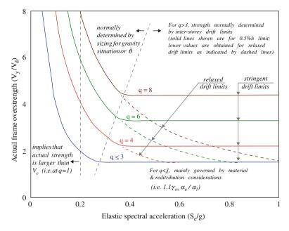
Fig. 5.7 Expected levels of lateral over-strength in moment frames
