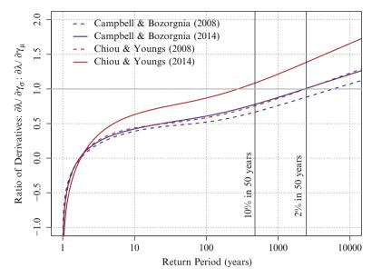
**Fig. 4.6** Ratios of the partial derivatives with respect to the logarithmic standard deviation and mean. *Vertical lines* are shown to indicate the commonly encountered 475 and 2,475 year return periods
