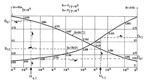
**Fig. 17.4** The normalized values of the variation of dynamic torsion modulus function  $(G, \text{daN/cm}^2)$  and torsion damping function (D %) of specific strain  $(\gamma \%)$  for sand and gravel samples with normal humidity obtained in Hardin and Drnevich resonant columns from NIEP (USA patent) (Marmureanu et al. 2010)
