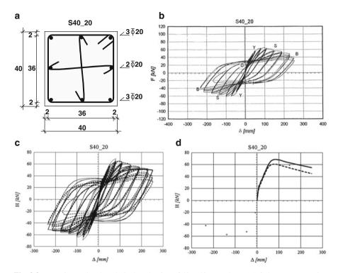
Fig. 8.8 Experimental and analytical evaluation of  $40 \times 40$  cm column (a) Column cross section (b) Typical force-displacement relation (c) Comparision of experimental and analytical results (d) Effect of material coefficient on the envelopes of force-displacement hysteresis
