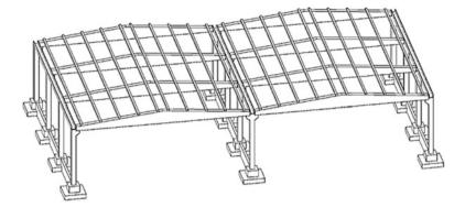
Fig. 8.1 Single story precast frame type structure
