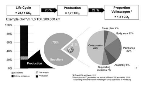
Fig. 23.2 Life cycle perspective: A car's CO<sub>2</sub> equivalents
