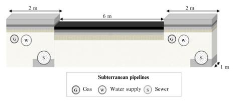
Fig. 22.1 The urban fabric: profile of the paved skin and subterranean pipelines under assessment
