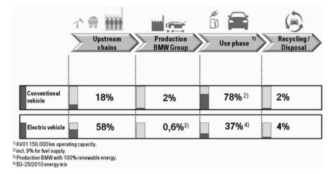
Fig. 24.1 Global warming potential [CO<sub>2</sub>e] results along the vehicle life cycle at BMW Group
