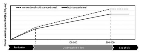
Fig. 23.3 Carbon footprint comparison: cold stamped steel vs. hot stamped steel
