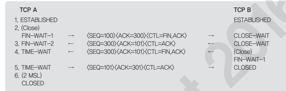
(Figure 51) General procedure for connection termination [1]
